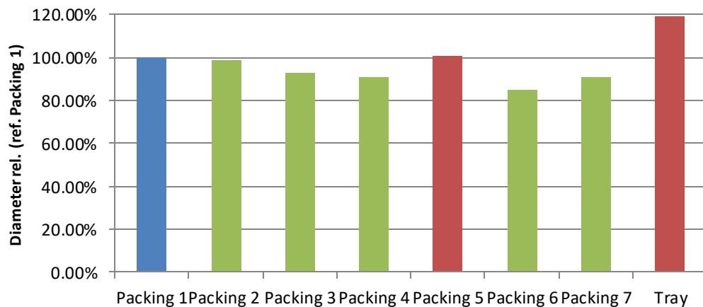
Figure 61. Diameter comparison for different packing using PACKING 1 like reference, for the feed gas with 3.5% of CO 2 and H 2 S.
