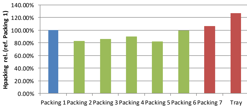
Figure 44. Bed height comparison for different packing using PACKING 1like reference, for the feed gas with 3% of CO 2 .
