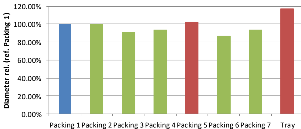
Figure 45. Diameter comparison for different packing using PACKING 1like reference, for the feed gas with 3% of CO 2 .
