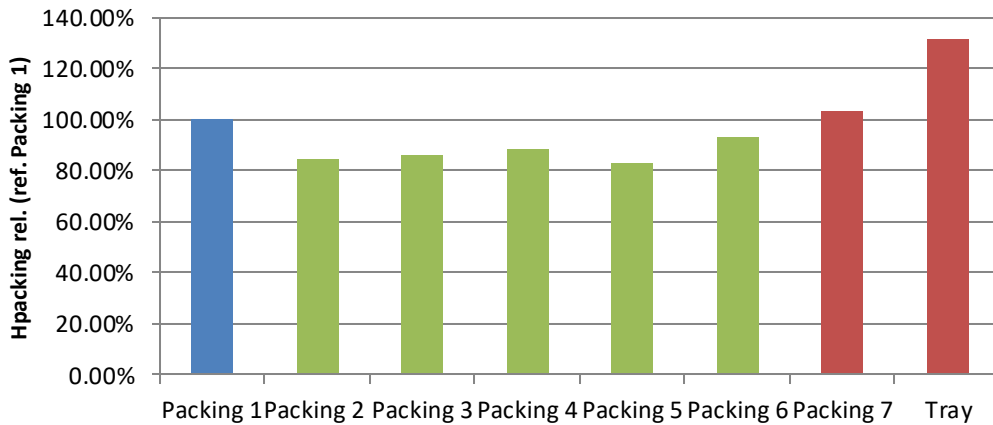
Figure 60. Bed height comparison for different packing using PACKING 1 like reference, for the feed gas with 3.5% of CO 2 and H 2 S.
